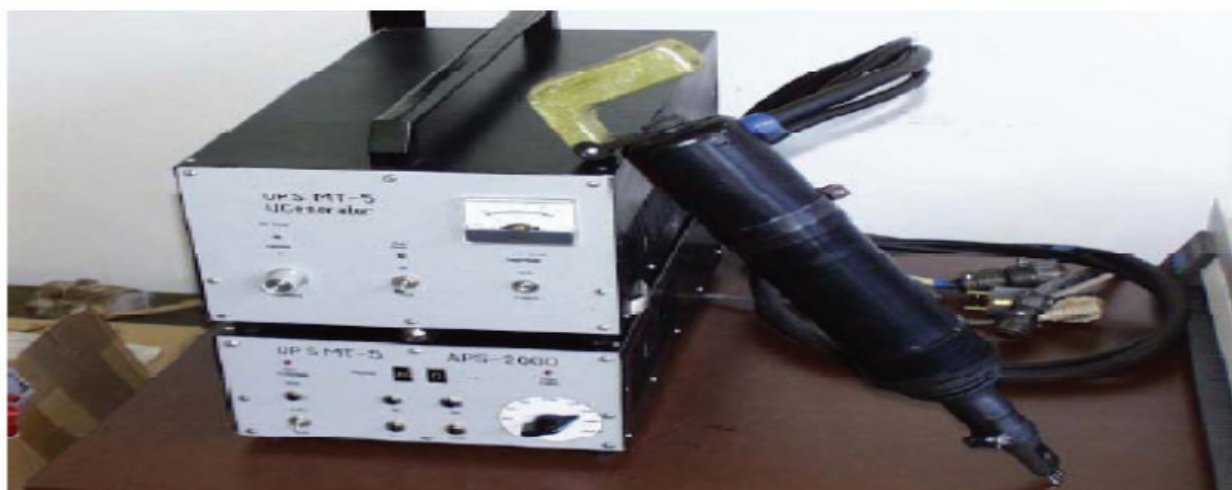
Fig.2 The 27 KHz ultrasonic impact treatment equipment.
